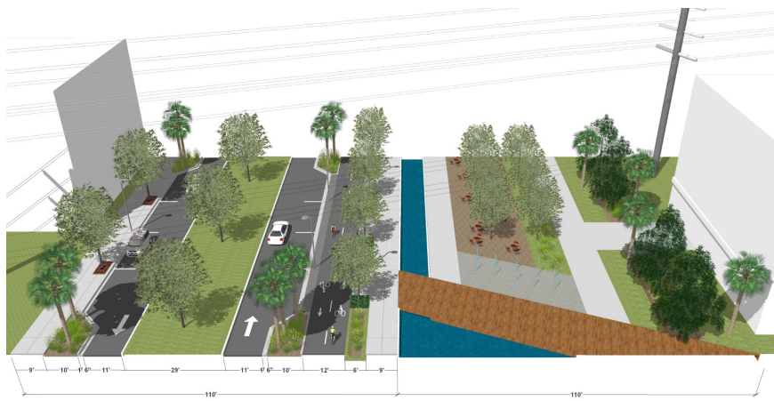
Initial street section showing single lane in either direction and wide median planted with street trees.
