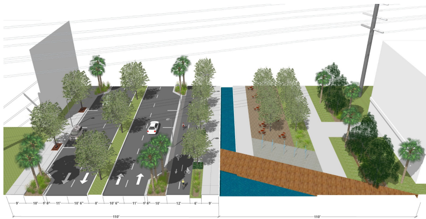
Potential long-term street section showing conversion to two lanes in each direction.
